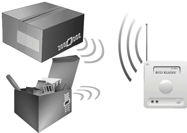
Figure 2. Schematic of operation on the RFID system.
